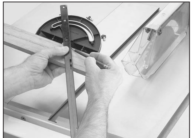
Figure 45. Example of marking miter line.
